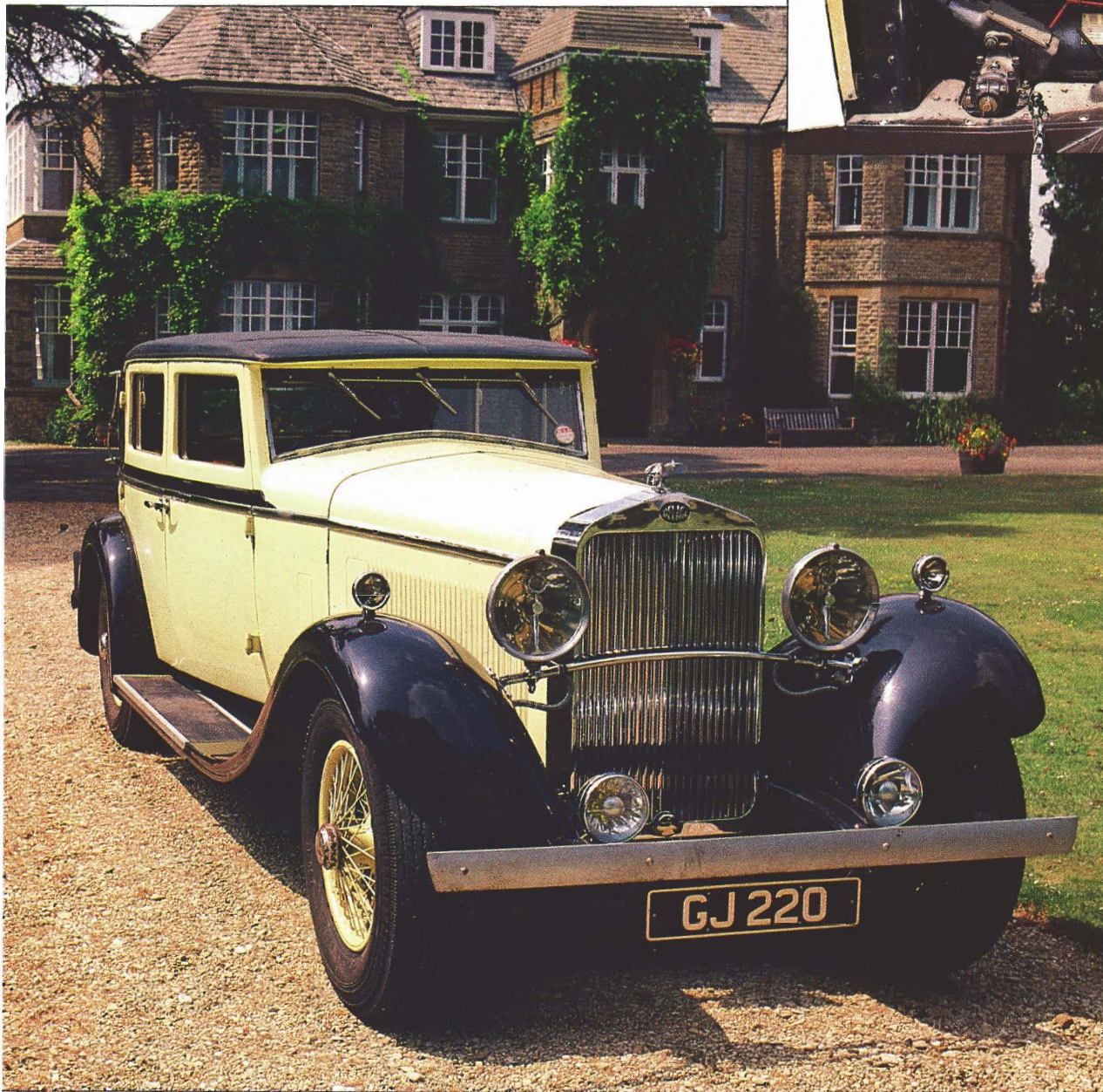
Above: The D8 was powered by an efficient eight-cylinder four-litre unit with five crankshaft bearings, which produced 120 bhp at the very start of its development. Even with the unaerodynamic coachwork fashionable at the time, the top speed was nearly 100 mph.
